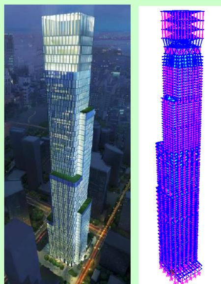
**Fig.10 Architectural rendering & structure model**
