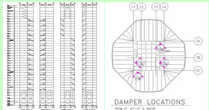
Fig.3 Boston 111 Huntington Tower and Damper Layout
